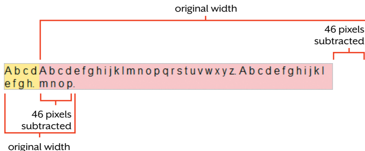
FIGURE 7.6 Both divs have 46 pixels subtracted from their widths in order to fit in the 500-pixel-wide box.
