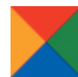
FIGURE 2.6 When a box has no width or height, each border creates the appearance of a triangle.
