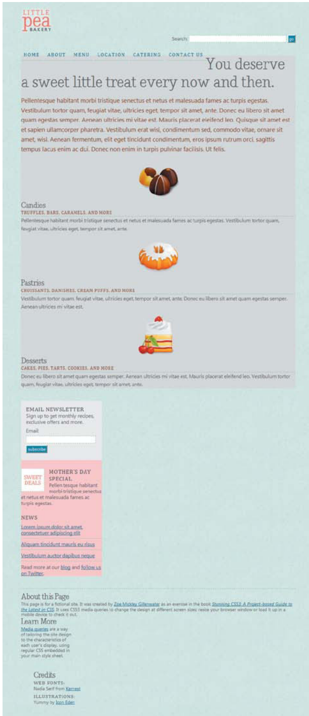
FIGURE 7.19 The layout is broken in browsers that don't support flexible box layout, such as IE 8.
