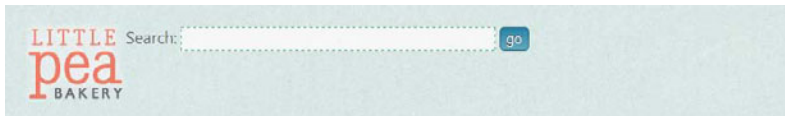
FIGURE 7.15 Now that the logo and the search form are children of a flexible box, they sit side by side.
