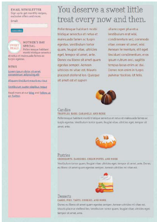
FIGURE 7.14 The two content divs stretch to the same height, because the children of boxes are given a box-align value of stretch by default.
