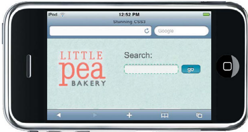
FIGURE 6.23 In landscape mode, the iPhone still shows only 320 pixels, zooming in so it fills the 480 pixels of width available.
